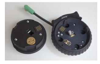
The tool is hold in position by a unique coupling with steel balls. This ultra-precise connection gives the tool changer an extreme high repeatability
