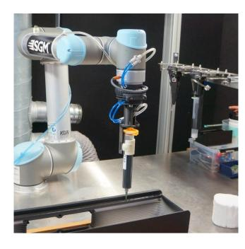
SGM Lights use a UR5 robot for assembling front panels for their spotlights.
