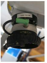
The robot can be programmed to change between tools. Tools are parked in docking stations. Manual operation is also possible
