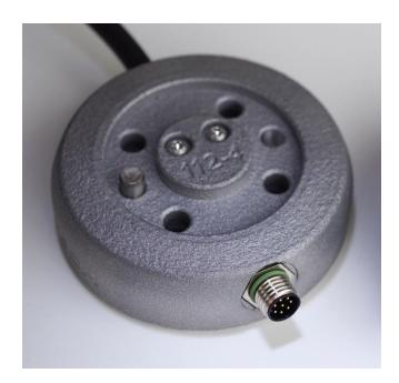
Smart adapter flange for small robots
