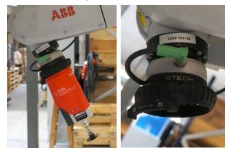
4TECH Adapter Flange makes it possible mount all tools designed for UR robots on robot arm with the smaller 40-4-M5 flange. The build-in tool connector socket makes electric connecting of power and signals easy
