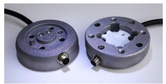
This new flange is made to fit tools on robot arms with smaller flanges. The flange has a build in electric socket that also makes it easy to connect the tool to the robot controller
