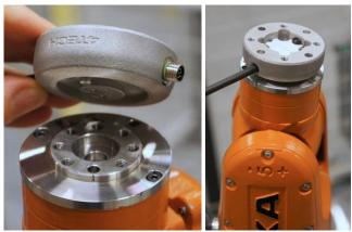
KUKA robot ready for Universal Robots tools
